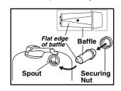
**CAUTION**: To prevent personal injury or property damage, the boiling chamber must be fully engaged prior to start-up.
