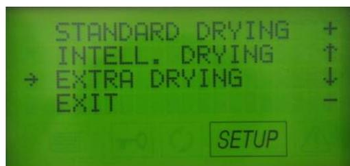
Once "EXTRA DRYING" is highlighted, press the START/STOP button to select that option. This will take us to the "EXTRA TIME" screen, from which we can add additional minutes to the end of the Bravo's standard 14 minute drying stage. To set the unit to maximum drying time, simply press the PLUS button until the top line of your display reads "EXTRA TIME: 15 MIN" as shown below:
