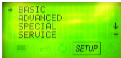
If Insert Password appears turn the main power switch OFF. To turn the password OFF press and hold the Setup button while turning the main power switch ON. The Insert password screen will appear. Press the Minus button 8 times, and then press the Enter button to confirm.
