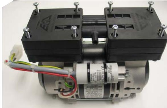
7. Now we can lift the head assembly off of the pump proper, maintaining orientation as shown below. Use both hands to prevent head sections from falling off while moving.
