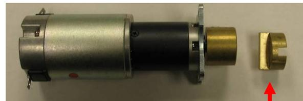
Remove the old motor through the opening in the bottom of the Bravo and install the new motor and coupling retained when old motor was removed. Reconnect the white and black wires making sure the white wire is connected to the terminal with the red dot.
