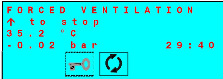
Push the ↑ key to interrupt the ventilation and open the door.
