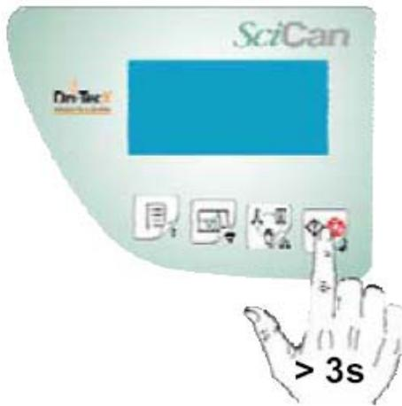
The operator can manually interrupt the cycle at any time by pressing the Start/Stop key for three seconds. This command generates an error code **E999** because the cycle did not finish correctly. Until it is safe to open the door, the unit will beep and the display will show:
