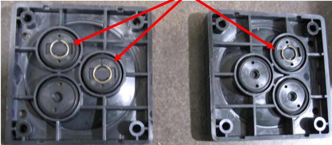
12. Remove all shutter-disks and o-rings (6 disks, 12 o-rings total). Each disk has two o-rings around its outer edge (one on each side), be sure to remove them all. Place two new o-rings on each new shutter-disk and set them in place, oriented the same as they were (as shown below).
