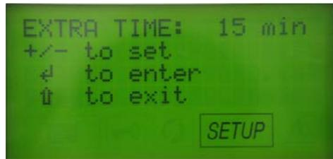
From here, keep pressing the PLUS button to increase the additional drying time up to a maximum of 15 minutes as before. When finished, press the START/STOP button. This will take us back to the list of cycle presets again:
