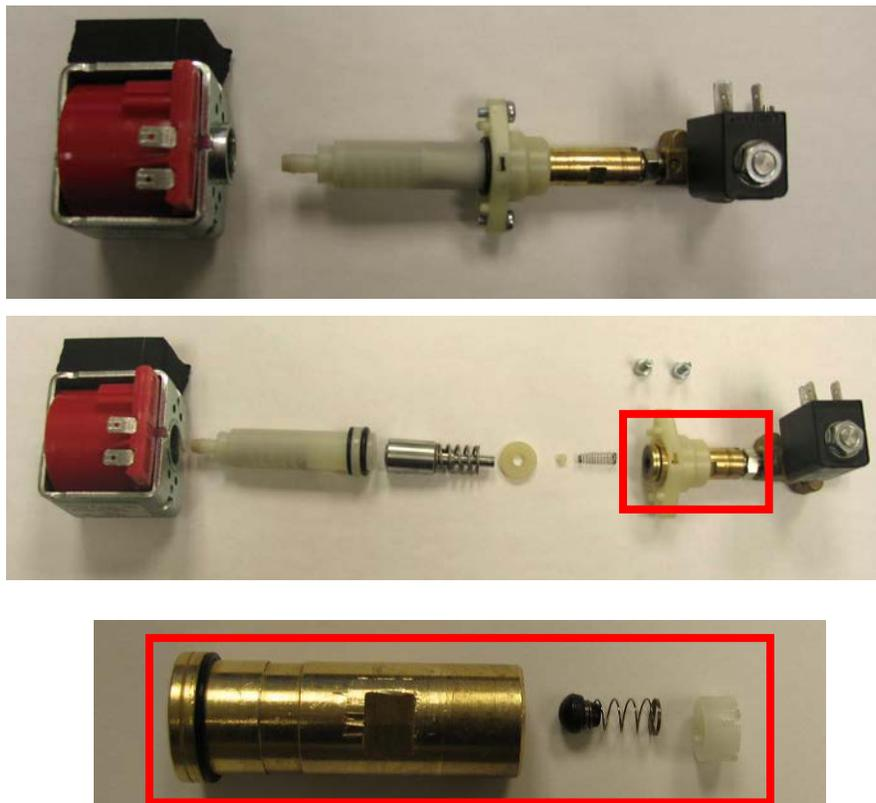
Reassemble pump and check for water flow through water pump (part #40000220000) & EV6 (part #40100370000)(water pump complete w/solenoid part #95509145). If water flow is good go to step 4.
