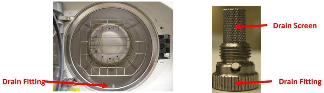
2. Check for excess moisture in the chamber. Make sure Bravo has 2 inches of clearance on the left side, right side and the top and 4 inches of clearance in the rear. Dry chamber and try another cycle.
