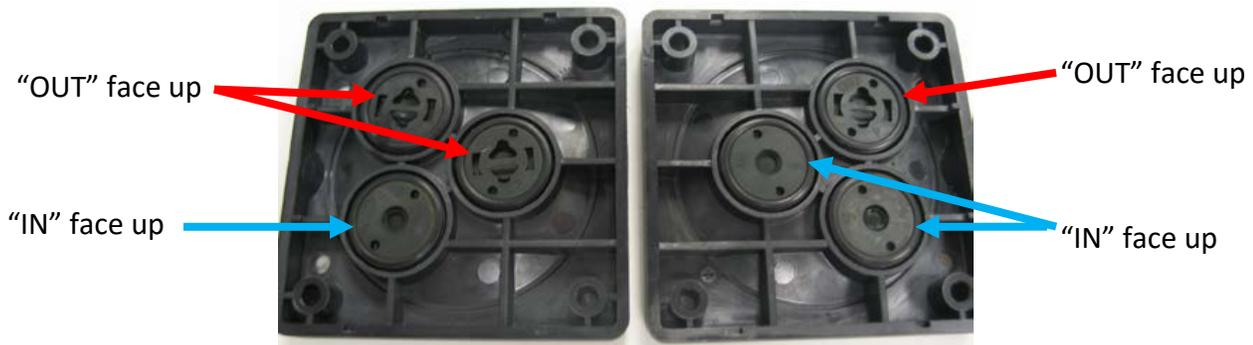
11. In some older style vacuum pumps, the shutter-disks used small c-clips to hold the shutters in place. If your pump has these older shutter-disks with c-clips, no need to worry, simply replace them with the new shutter-disks provided with your rebuild kit.
