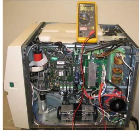
To access the Steam Generator safety thermostat, remove the six screws holding the condenser coil cover.
