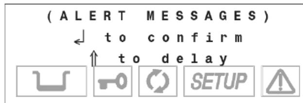
Push the ← key to confirm the recommended “routine” maintenance operation has been performed.
