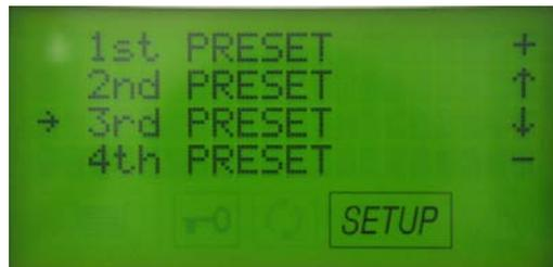
Now we are almost finished, both of your Bravo's Wrapped cycles have been set to maximum drying time. To exit the Menus, simply press the MENU button 3 times, until your screen looks like this:
