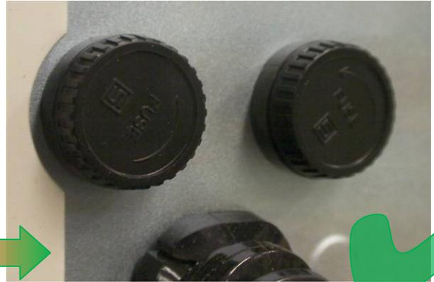
When replacing fuse holders connect white & blue wires to one fuse holder and black and brown wires to the other fuse holder.
