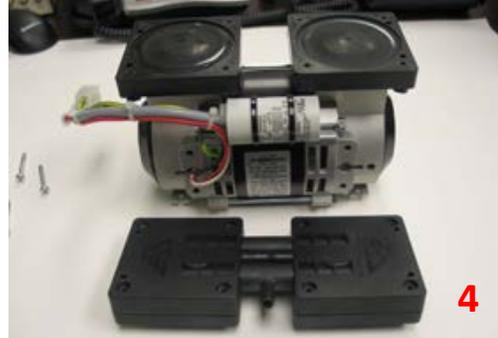
8. Looking downward at the head assembly you just removed, note the two input/output posts in between the two square heads. The output post will likely be out of view as shown below. For ease of recognition, rotate the post into view as shown below. Both direction arrows will now point in the same direction (away from you).
