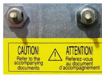
**Note: The Steam Generator Safety Thermostat (part #97730011) is located on the left and the Band Heating Element Safety Thermostat (part #97730010) is located on the right when facing the rear of the Bravo. A small screwdriver or instrument will be required to reset the original style thermostat.**
