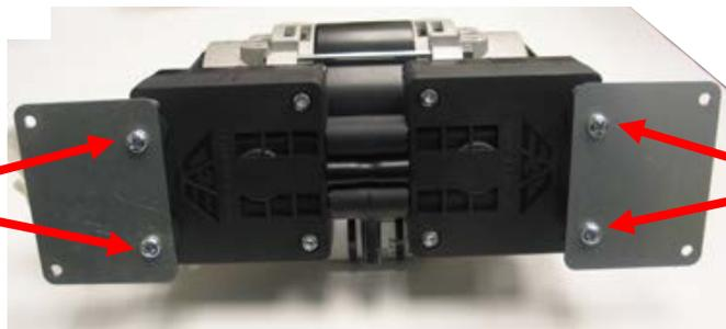
4. Next, remove the four rubber mounting posts from the base of the pump (two on each side).
