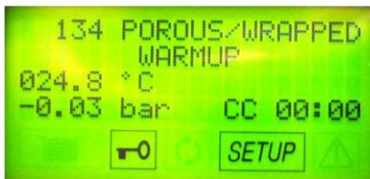
**Note: If you wish to return the Bravo to its normal operating mode you will need to return to the Test Cycles screen and turn the Test Cycles OFF.**
