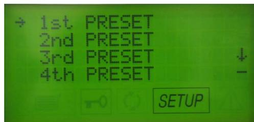
Now we want to move down the list and select "3<sup>rd</sup> Preset". Simply press the MINUS button twice to highlight "3<sup>rd</sup> Preset" as shown below, and then press the START/STOP button.
