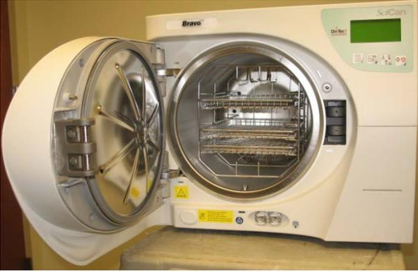
Clean the door gasket and front of chamber with a clean cotton cloth soaked in a weak solution of water and vinegar. Dry the surfaces and remove any residue before using the device.
