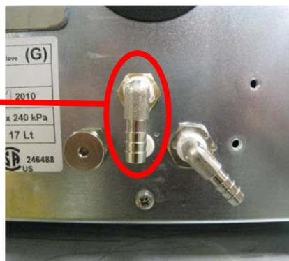
Connect the drain tubing to the elbow fitting using a tie wrap and install the plastic drain tube holder underneath the rear of the Bravo, below the elbow fitting. Feed the drain tubing through the holder. Mount the second drain tube holder underneath the front of the Bravo below the H2O drain sticker. Make sure the orange plug is installed into the end of the drain tubing.
