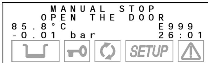
Finally when the door is opened you will be asked to **Reset** the device by the following message:
