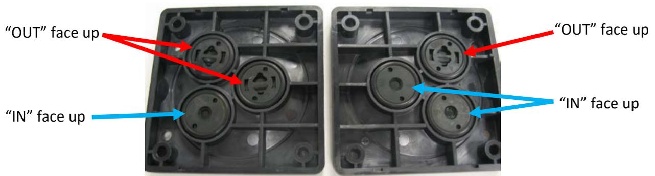
13. Now we can address the other section of the head units that we removed in step 9. Make sure there are no o-rings left behind from the old shutter-disks in any of the six round fittings
