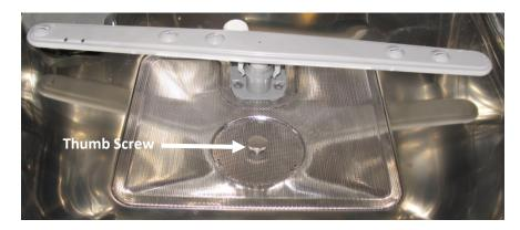
Check the fixed screen, sump for debris. Remove the Phillips screw from the center of the screen and the two Phillips screws holding the lower wash arm mount. Removed the fixed screen, sump and clean as needed. (Fixed Screen, Sump part #01-113387S)
