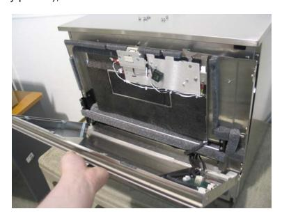
At this point, the only thing attaching the door cover panel to the Hydrim is our touchscreen interface assembly. We can leave the machine as-is and proceed from here with the step after this one, but if you'd like to make things easier (space-wise), we can remove the touchscreen assembly from the door cover panel by removing the nuts shown below:
