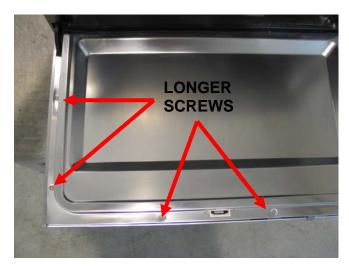
With the above seven total screws removed, you may now lower the door panel towards you exposing the latch mechanism. There may also be a piece of carpet-like insulation behind your door panel (not shown in my picture), set it aside for now.
