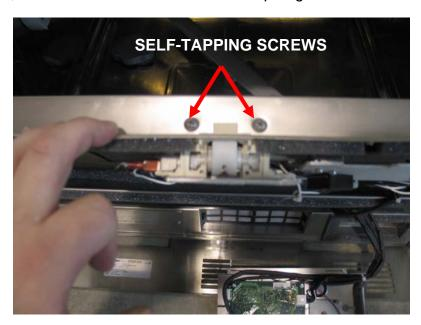
Next, remove the last mounting screw on the right side of the panel as shown below:
