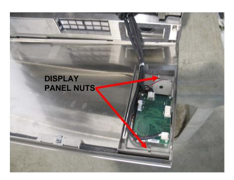
Now we are ready to remove the old door latch mechanism from your machine. For the purposes of this repair, we will be replacing the entire panel shown below. This will make the repair easier and will ensure that we replace any and all parts that could be causing the customer's "door open" alarm messages. To start, remove the two screws from the top edge of the door as shown below.
