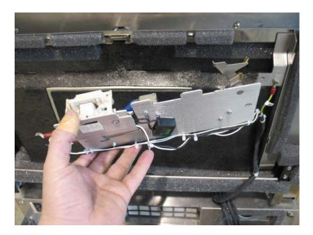
Flip the panel over so that we may access the rear side of it. Remove the six wires connected to the two microswitches and the solenoid from the rear of the panel. The wires and connections are labeled on the following image for your reference during re-assembly:
