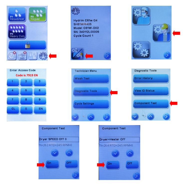
When testing the dryer speed as you keep touching the ON button the RPM will keep increasing. Speed will go from 0 to 31.
