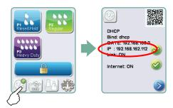
3. Type the IP address displayed on the touchscreen into the browser of any web enabled device to access your unit's web portal. When the Network icon is active (for example when sending email) it will turn green.
