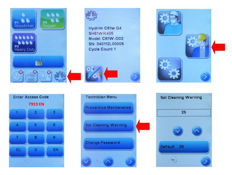
The reminder frequency for the chamber cleaning can be set to 25, 50 or 100.
