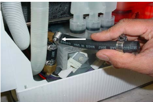
Push the assembly in so wires and hose are accessible where valve block was removed.
