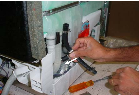
Push the assembly in so wires and hose are accessible where valve block was removed.
