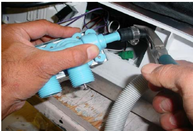
Connect black hose to valve block
