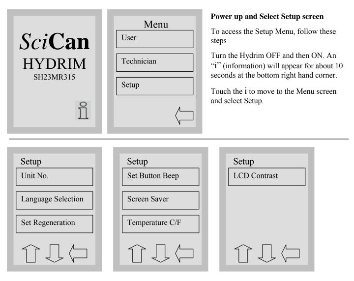
The Setup Menu consists of seven choices as shown above. Using the up and down arrows to move through the choices, touch the desired option to select it. For more detail on each Setup Menu option, refer to the following sections.
