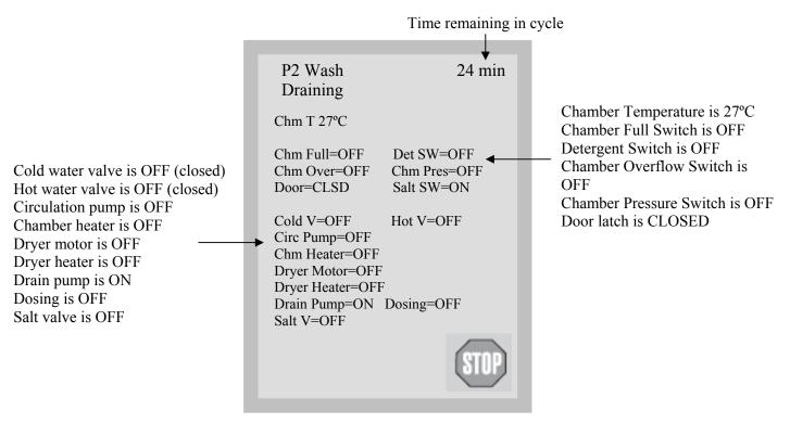
The Debug cycle should be used when troubleshooting to view the IO status of components.
