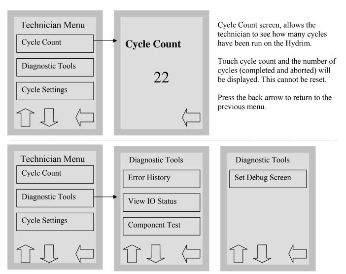
The Diagnostic Tools menu consists of four choices. Up arrow pressed, change to previous Diagnostic Tools screen. Down arrow pressed, change to next Diagnostic Tools screen. Press the back arrow to return to the previous menu.
