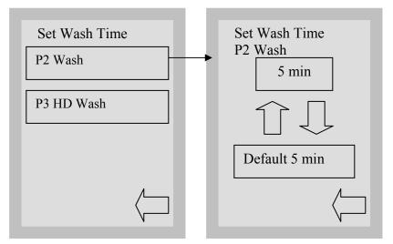
P2 & P3 wash times Min Value 5 min – Max Value 15 min Default Values P2 – 5 min & P3 – 9 min
