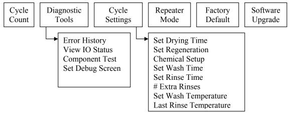
To access this menu, turn the unit OFF and ON. There is an "i" in the lower right hand corner of the screen for about 10 seconds. Touch the "i" to get to the menu screen. Touch Technician.
