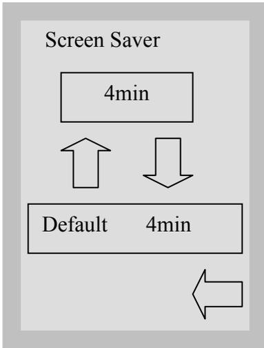
The user can adjust the time that elapses before the screen goes into screen saver mode. Touch the up and down arrows to select the desired screen saver setting. The default is 4 minutes. Touch the back arrow to return to the previous menu.
