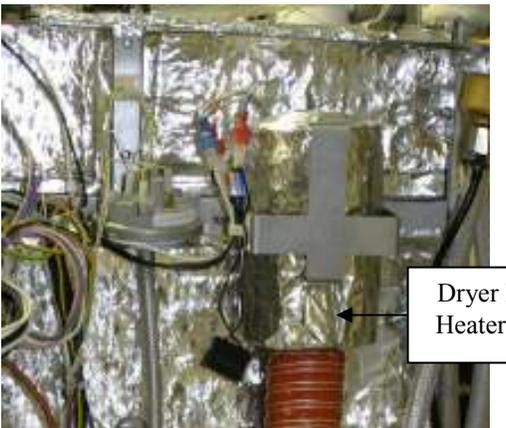
Remove top cover and right side panel to access the Dryer Motor and Heater Assembly.
