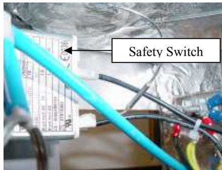
Remove filter screen from inside chamber and unclip Safety Switch Probe from Heating Element.
