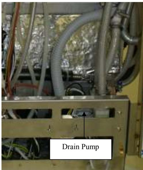
Remove top cover and right side panel to access the Drain Pump.
