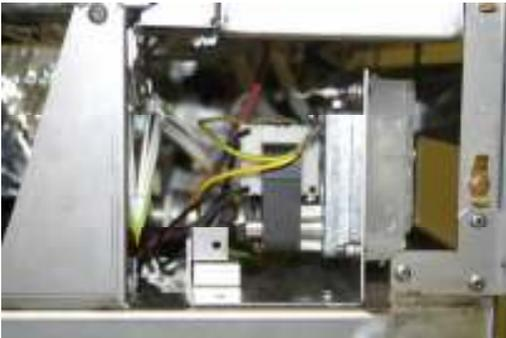
The Dosing Pump is located behind the cover below the front door. Remove screw from top center of cover and locate the Dosing Pump on the right side. Remove two mount screws to access the Dosing Pump. **Dosing Pump Part # 21972.01**
