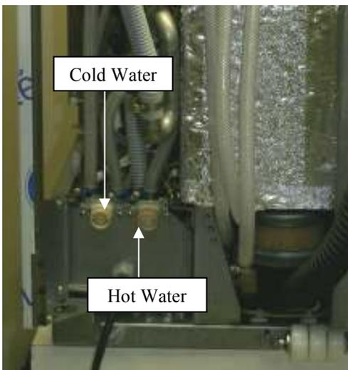
Remove the top and rear covers to access the Cold & Hot Water Inlet Valves. The dual valve is for cold water and the single valve is for hot water.
