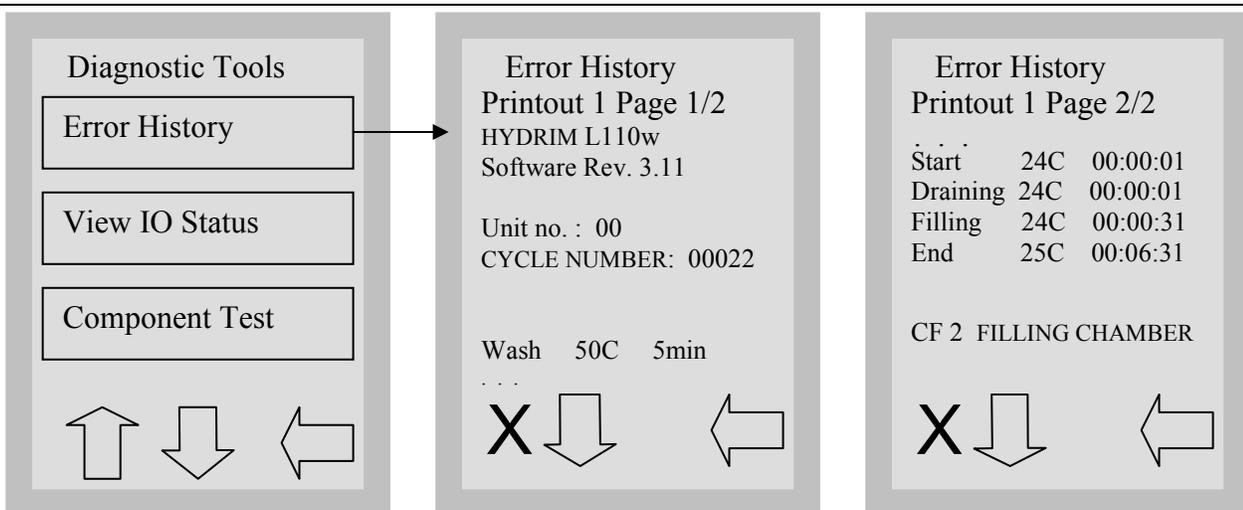
Error History screen, allows the user to see the last four errors. Press the down arrow to move to the next page / error. Press the X in the lower left hand corner to clear the error history. There must be 4 errors stored to clear the error history and the last error will remain.
