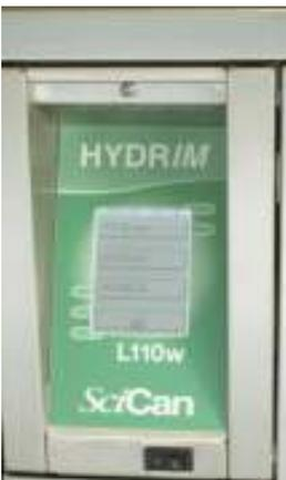
Remove the screw above the touch screen and open door. Disconnect I/O Board and Logic board from Touchscreen, replace the touchscreen and re-connect the boards in reverse order. Close the door and re-insert the screw above the touchscreen.
