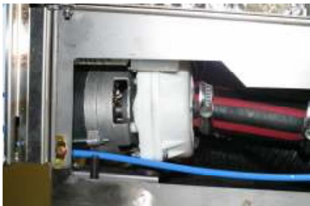
Remove top cover, rear and left side panels to access the Circulation Pump.
