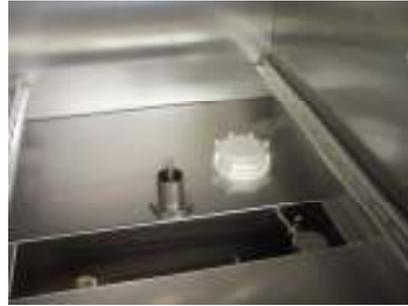
After salt has been added to the unit, the softening salt indicator will initially indicate salt needed. The indicator will turn off when the salt solution has become sufficiently concentrated.
