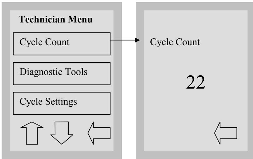
Cycle Count screen, allows the technician to see how many cycles have been run on the Hydrim.
