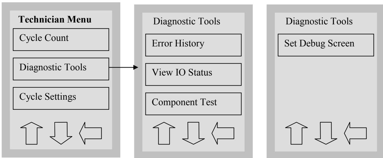
The Diagnostic Tools menu consists of four choices. Up arrow pressed, change to previous Diagnostic Tools screen. Down arrow pressed, change to next Diagnostic Tools screen. Press the back arrow to return to the previous menu.
