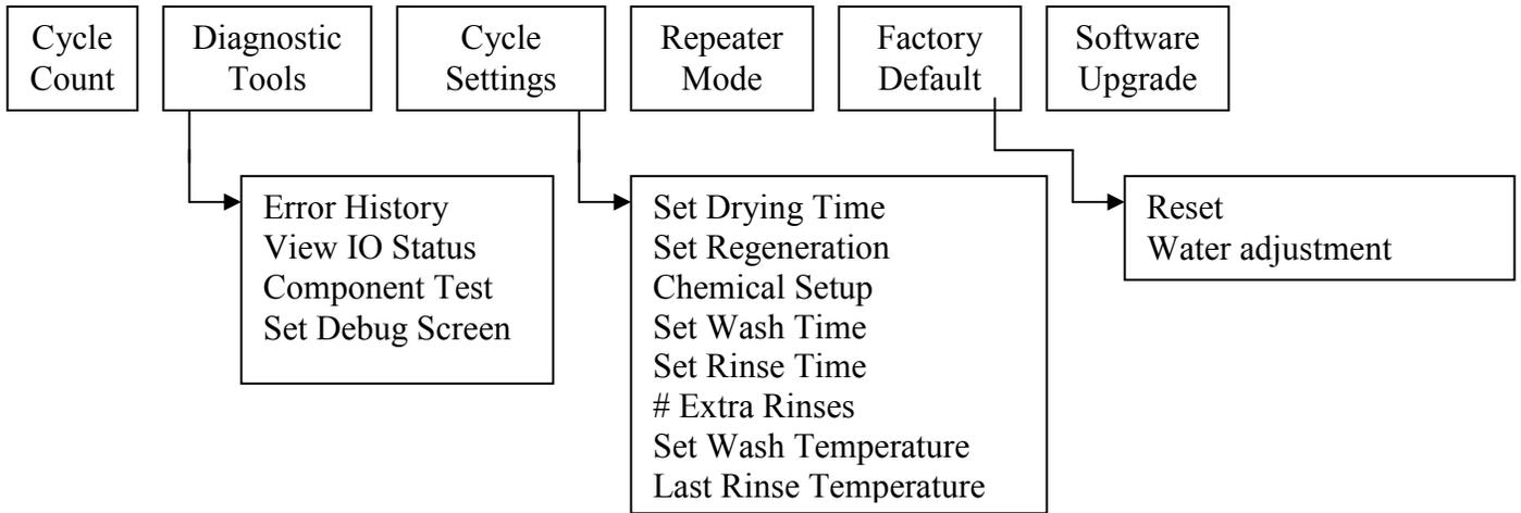
To access this menu, turn the unit OFF and ON. There is an “i” in the lower right hand corner of the screen for about 10 seconds. Touch the “i” to get to the menu screen. Touch Technician.
