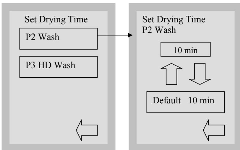
The drying time for P2 and P3 can be set independently.
