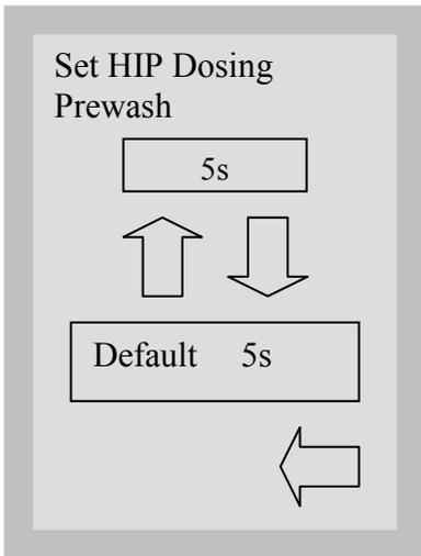
Use the up and down arrows to select the desired dosing setting for the cycle selected. (Do Not change default setting unless directed by SciCan)
