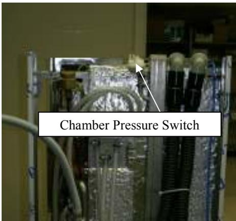
Remove the top and rear covers to access the Chamber Pressure Switch.
