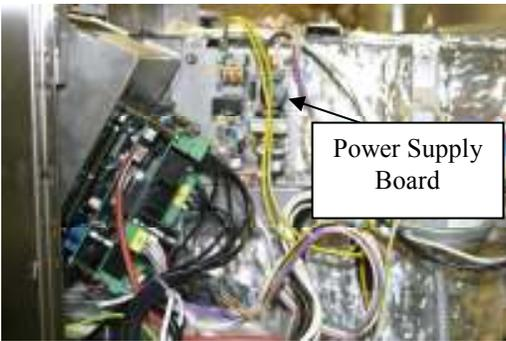
Remove top cover and right side panel to access Power Supply Board.
