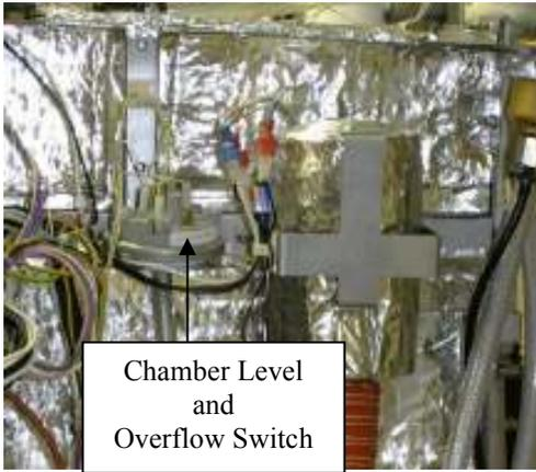
Remove top cover and right side panel to access the Chamber Level and Overflow Switch.
