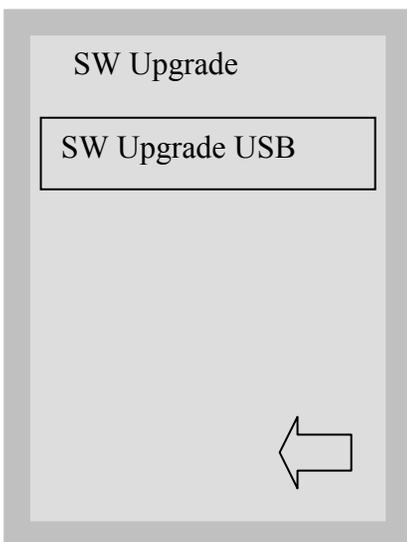
SW Upgrade USB button pressed, start SW upgrade procedure. This option allows technician to upgrade software by using a USB Data Logger and files stored on a USB Memory Stick.
