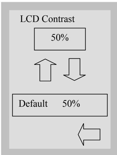
The user can change the contrast on the display. Touch the up and down arrows to select more or less contrast on the display. The default is Touch the back arrow to return to the previous menu.
