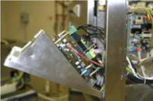
Remove the screw above the touch screen and pull out the door to access the IO Board and Logic Board. Replace as needed.
