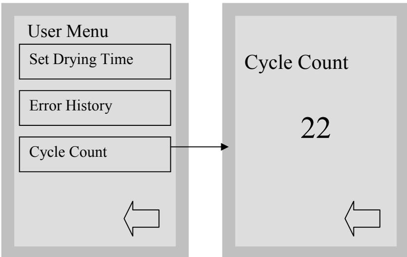
This allows the user to see how many cycles have been run on the Hydrim. Touch cycle count and the number of cycles (completed and aborted) will be displayed. This cannot be reset. Touch the back arrow to return to the previous menu.
