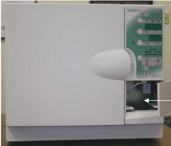
Open door and insert hand to access door solenoid
