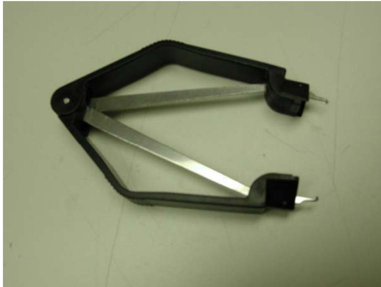
There are two small slots on two corners of the socket. Insert the remover tips in the two slots squeeze the black arms and pull the chip out.
