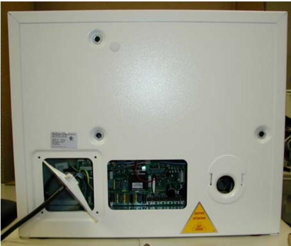
When reinstalling the cover reconnect the exhaust fan plug to the 2-pin connector marked fan and the rear fan assembly to PL 34. **Note: Not all Quantims have a rear fan assembly.** Also reconnect the exhaust tubing if used.
