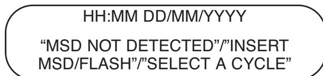
Messages “MSD NOT DETECTED”, “INSERT MSD/FLASH” and “SELECT A CYCLE” will rotate in sequence and not all appear at the same time.
