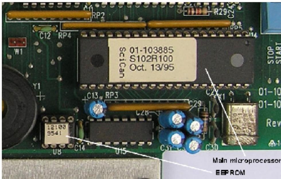
The microprocessor and EEPROM devices are a matched pair set. These devices are supplied together and must be installed together. Any attempt to substitute either device on its own will result in a continuous beeping tone.
