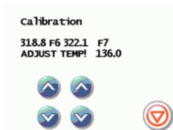
**IMPORTANT NOTE:** When the initial pressure and temperature readings have been adjusted, and to ensure equilibrium of the calibration, compare the measured chamber pressure (PPP.P) and the calculated chamber pressure (TTT.T) displayed on the LCD. They should be within 1 kPa of each other during equilibrium.
