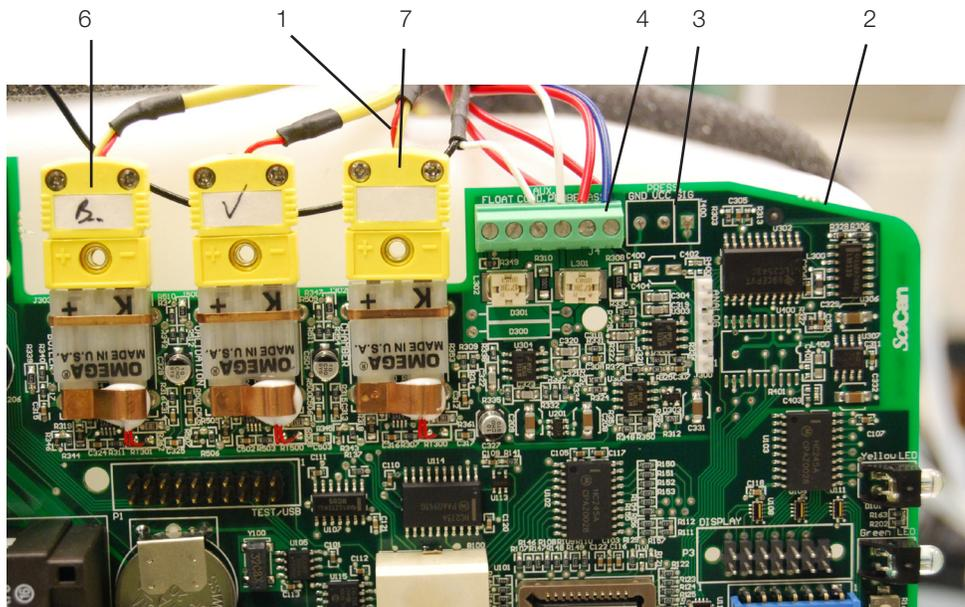
1. Chamber thermocouple leads
