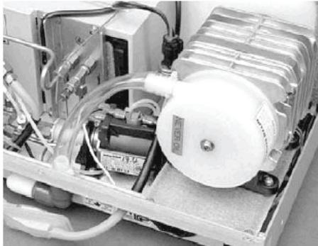
The MEDO Compressor draws air through the cylindrical air filter at the back of the unit and into the compressor, then pushes the air through the bacteria-retentive air filter and check valve into the steam generator.
