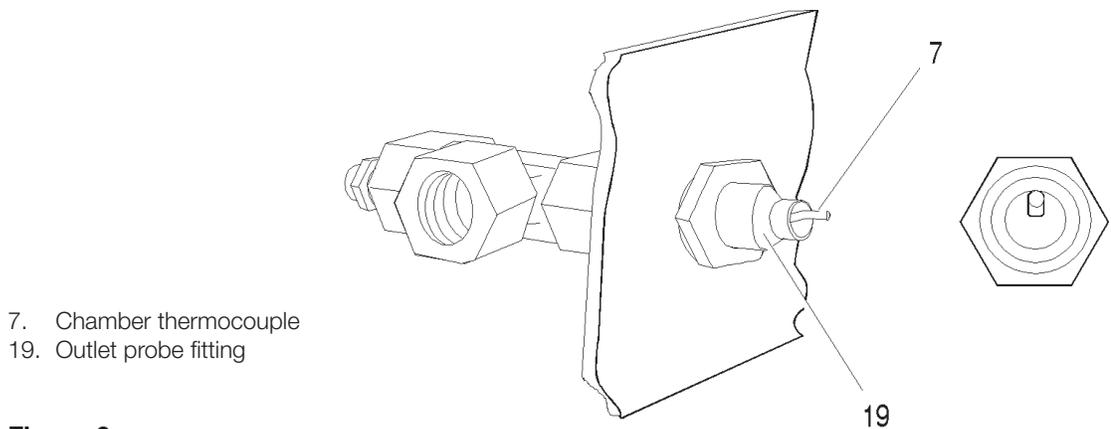
7. Chamber thermocouple
