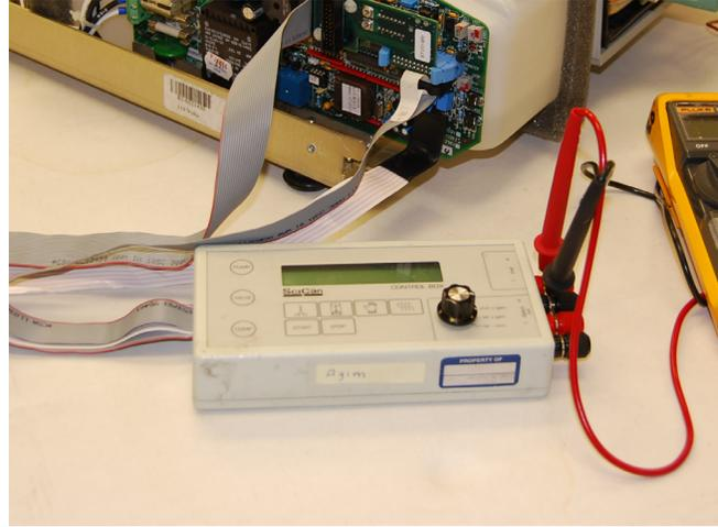
The Control Box (5) is a service tool that allows a technician to operate the unit while it is being serviced. There are two kinds of Control Boxes you may encounter: one uses toggle switches, the other uses a membrane keypad arrangement similar to the keypad on the unit.
