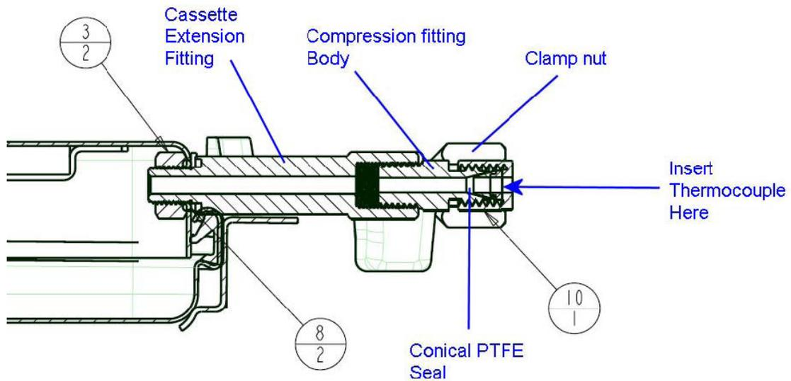
**Figure 8.** Temperature fitting cut-away
