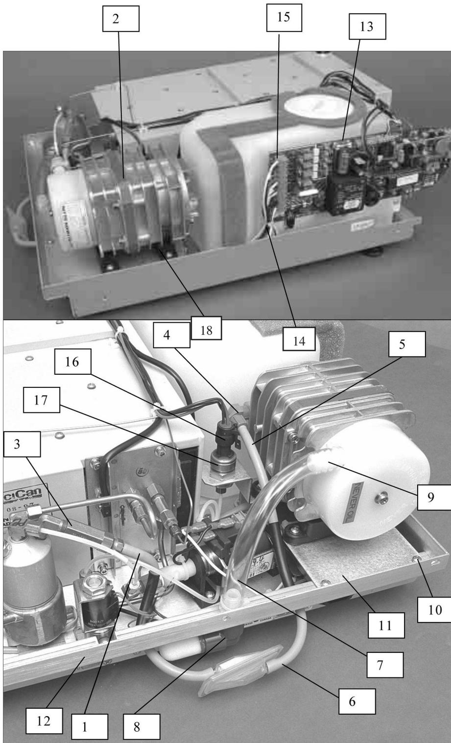
1. Rubber Tube (cylindrical air filter only)
