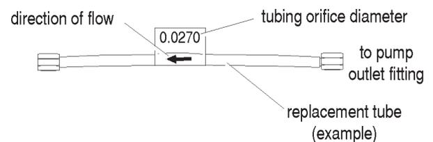
Single pump tubes are available in a large number of diameters from 0.0210" diameter to 0.0290" diameter in 0.0005" increments.
