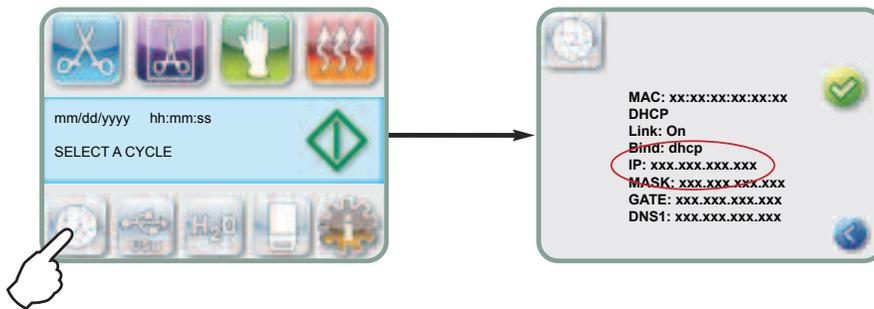
3. Type the IP address displayed on the touchscreen into the browser of any computer connected to the same network as the STAT/IM to access your unit's web portal. You will know that an IP address has been assigned when the red X over the Network icon disappears.
