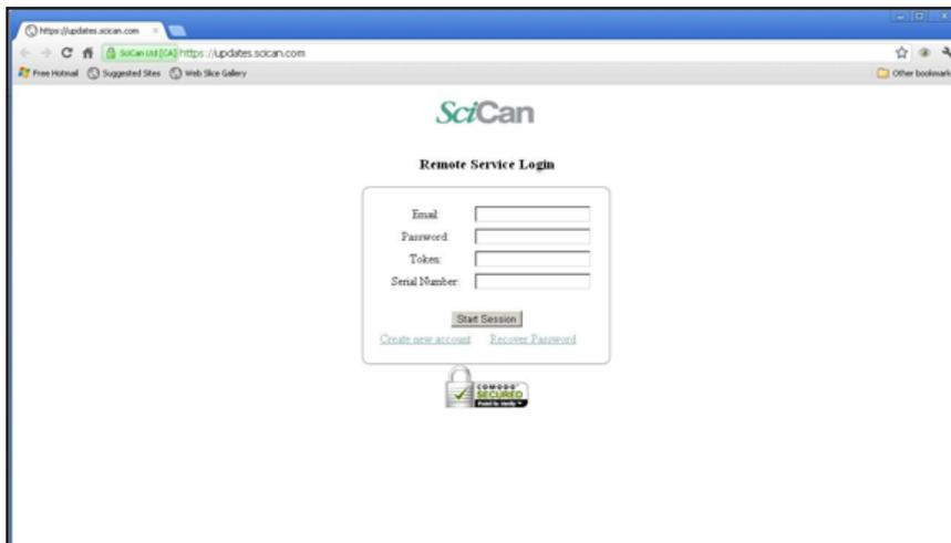
With a valid user name, password and token, a technician can remotely access the STAT/M G4 unit's web portal page.
