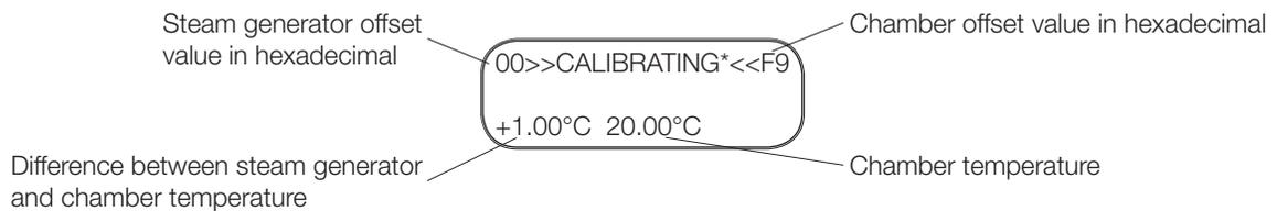
3. To start a steam generator (self-calibrating) cycle, **press and hold** the UNWRAPPED cycle button on the control box and press the **START** button. An asterisk \* will appear next to the message 'CALIBRATING'.
