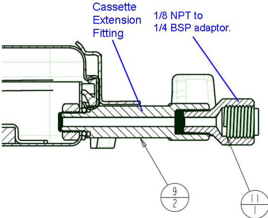
**Figure 9.** Pressure fitting cut-away
