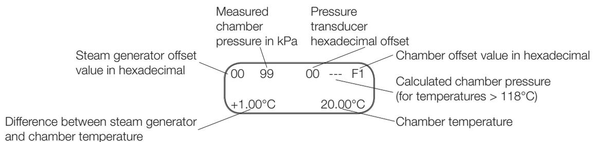
3. To start a steam generator (self-calibrating) cycle, **press and hold** the UNWRAPPED cycle button on the control box and press the **START** button. An asterisk "\*" will appear next to the steam generator offset value.
