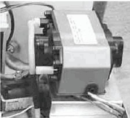
The THOMAS (or SciCan) Compressor draws air directly into the compressor from inside the unit and then pushes the air through the bacteria retentive filter and check valve into the steam generator.
