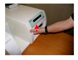
6. Push this tab to the left to unlock the LCD/keypad from the cover.
