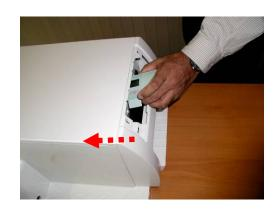
Release the cover retention clip by reaching inside the cover though the LCD opening and lift up on the tap located on the left most side of the opening. Slide cover forward.
