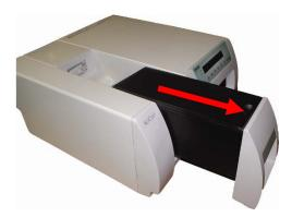
Remove the water filter or water bypass cartridge (if the unit is using distilled water) from the reservoir area.
