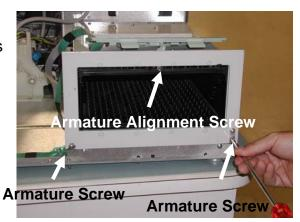
Armature is mounted on 2 rails which will allow the Armature to slide easily. Slide Armature forward and remove using two hands. There are no connections to the Armature.
