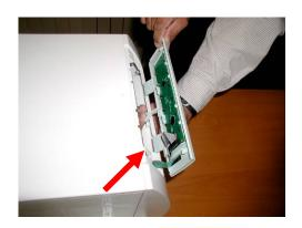
Place the LCD/keypad on top of the armature so that it is out of the way as you remove the cover.
