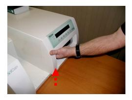
6. Push this tab to the left to unlock the LCD/keypad from the cover.
