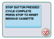
When the automatic 60-minute drying stage is finished the display reads:
