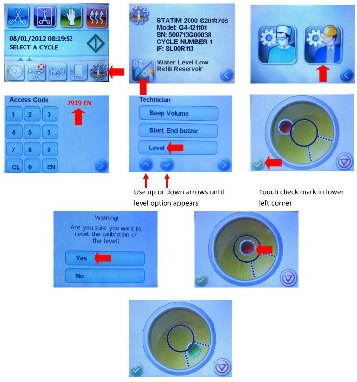
Adjust leveling legs until bubble level is in the lower right quadrant and turns green.
