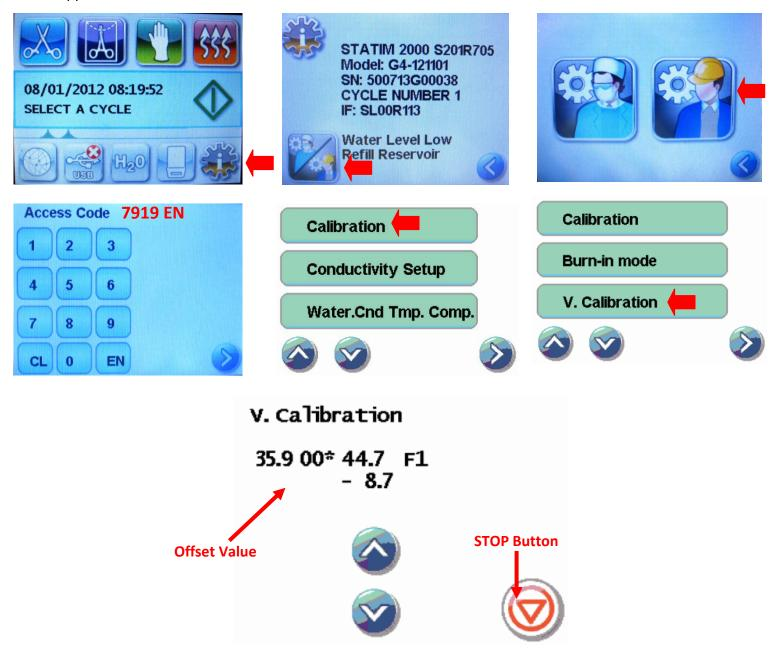
The calibration cycle will take approximately 6 minutes to complete. Allow the self-calibration cycle to complete. The temperature within the cassette will rise to sterilization temperature. Wait until the sterilization phase of the cycle ends automatically. The offset value in the upper left-hand corner of the display may have changed to a new offset value. Press the **STOP** button when finished.
