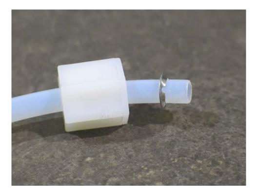
5. Then slide the small plastic washer onto the tubing, just as you did with the metal washer, wide end first.
