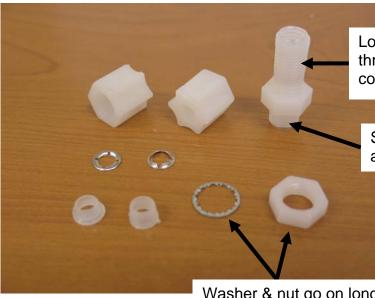
Long threaded end goes through top of the lid for condensing coil
