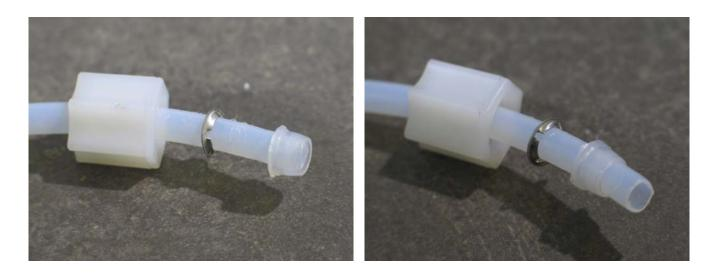
6. Now insert the assembled tubing into the threaded fitting on top of the waste bottle lid. As you screw down the large nut, the washers on the tubing will secure themselves, creating a tight seal at the bottle.
