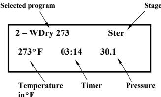
Example 3: The screen display showing a process that has failed due to temperature drop during the sterilization stage of program No.3.
