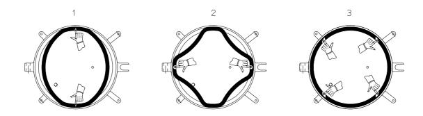
Pull off the gasket from the door groove and install the new gasket referring to the drawings as above points 1, 2 and 3.
