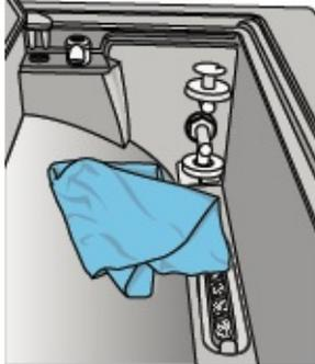
Wipe the reservoir's surfaces using OPTIM wipes or a clean, lint-free cloth dampened with water.
