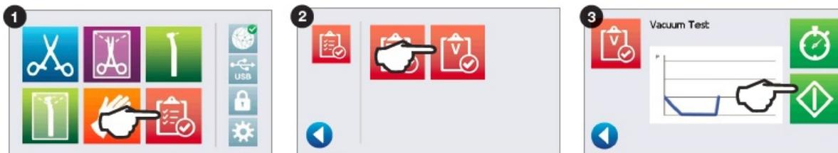
Running a vacuum test can take a minimum of 45 minutes. When the test is complete, the screen will display a CYCLE COMPLETE message. If the test has failed, see Troubleshooting.
