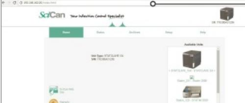
Type the IP address displayed on the touchscreen into the browser of any web enabled device to access your unit's web portal. To set up your web portal, follow the instructions available on the portal's **HELP** tab.
