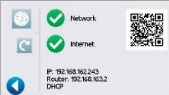
The connectivity screen displays information about your STATCLAVE's internet connection, including its IP address.
