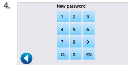
Using the keypad, assign a PIN of up to four digits. Press **EN** to save.
