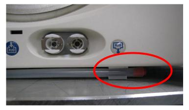
Note: If you are on manual fill, please fill the clean reservoir at this point with Distilled Water and proceed to Section 4. If you are on Autofill, please proceed to section 3 below.
