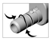
• Firmly squeeze the 0-ring between your thumb and index finger so that it forms a loop.
