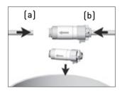
Replace the air filter and reconnect the air hose (a, b).
