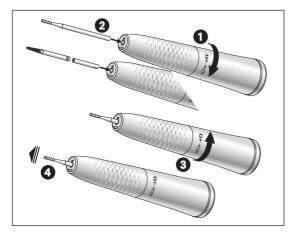
Straight handpieces Inserting the rotary instrument
