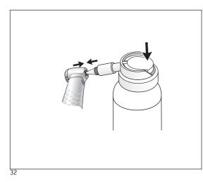
Lubrication of the chucking system WK-93, WK-99
