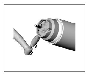
Lubrication of the chucking system
