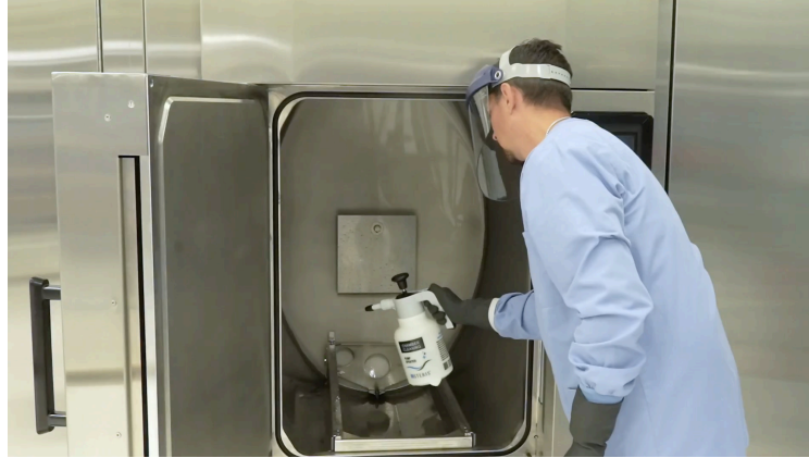
Figure 3-7. Spray Chamber with Diluted Cleaning Solution
