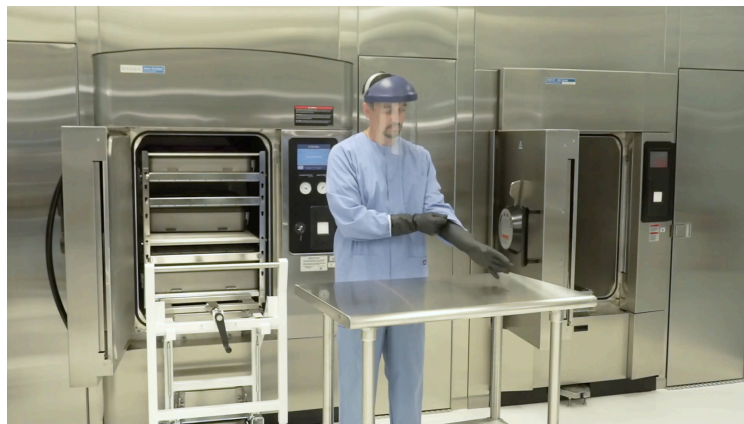
Figure 3-6. Required PPE for Cleaning
